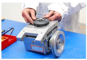
Place the new seal (108414PA002) in the intermediate flange and press it firmly in place.
