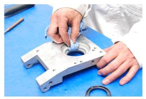
Thoroughly clean the cavity that houses the oil-retaining ring.
