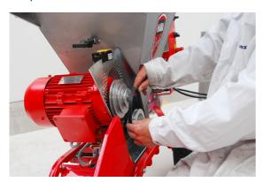
Now fit the V-belt (108414BP002) back on the pulleys.
