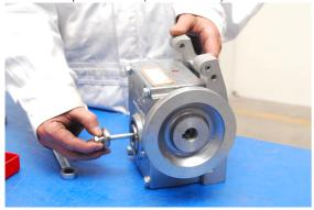
Fit the greased spindle back in the reduction drive and tighten it in place with the bolt and large washer.
