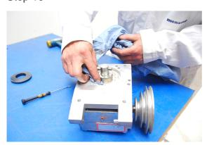
Thoroughly clean the cavity in the reduction drive that houses the seal (108414PA002).
