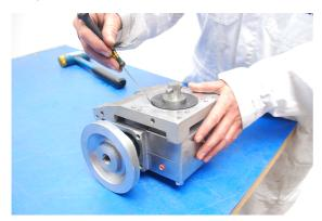
Place the reduction drive on a workbench with the side with the seal (108414PA002) facing up. Use a small screwdriver to remove this seal.
