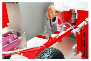
Loosen the four socket-head screws that attach the reduction drive to the stainless steel hopper. There are two socket-head screws on each side.
