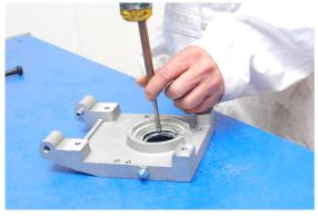
Now carefully tap the oil-retaining ring (108414BP005) out of the intermediate flange. Use a drift punch and hammer. Caution: tap it out carefully.
