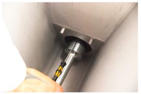
Greasing the seal. Position a small screwdriver between the seal (108414PA002) and the stainless steel hopper. Fit the grease pump to the grease nipple and pump several strokes.
