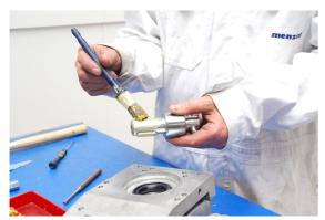
Grease the spindle MC3V (108402AS007).
