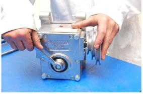
Remove the bolt from the spindle MC3V (108402AS007).
