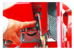
Now fit the handle for the V-belt tensioner back on the machine. Ensure that the lip of the tensioner rests on the motor base plate.
