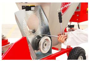
Loosen the bolt for the pulley guard. Move the pulley guard downwards.
