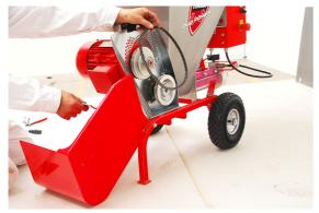
Remove the V-belt (108414BP002) from the pulleys. This is done by moving the handle down, which brings the pulleys closer together.
