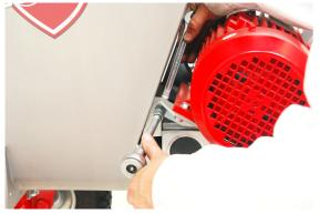
Loosen and remove the nut and bolt for the motor base plate.
