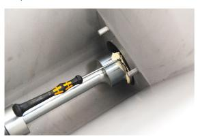
When grease appears at the seal (108414PA002) on the inside of the stainless steel hopper you have applied enough grease. Please note that this procedure must be repeated annually.
