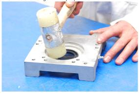
Use a hammer to carefully tap the oil-retaining ring into the intermediate flange.
