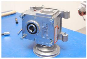
Fit the intermediate flange back on the reduction drive and tighten the four long mounting bolts.
