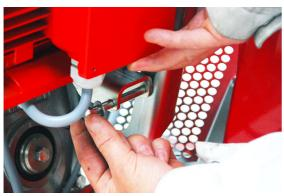
Fit the bolt with washer back in the handle of the V-belt tensioner and the motor base plate. Do not overtighten the bolt, because the handle must be free to turn.
