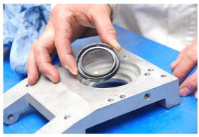
Fit the new oil-retaining ring (108414BP005) in the intermediate flange in the proper manner.
