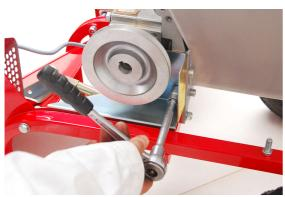
Also loosen the bolt for the bottom guard.
