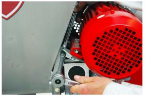
Tighten the mounting bolt with washer that secures the motor base plate.
