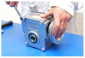
Loosen the four bolts that attach the intermediate flange to the reduction drive.
