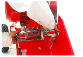
Loosen the bolt that holds the handle of the V-belt tensioner.
