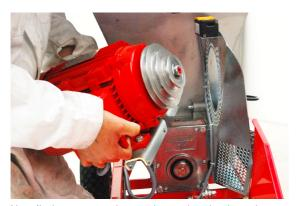
Now fit the motor and motor base plate back on the machine.
