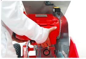
Now remove the motor and motor base plate from the machine.
