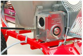
Now fit the reduction drive (108412BP014) back in the right place on the machine and tighten the four socket-head screws.
