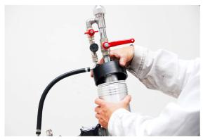
Unscrew and remove the front union nut (108401PA003), including the spraying section, from the repair gun.
