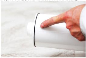
Press the O-ring (108401BP003) firmly against the lip of the cartridge to prevent any air leakage.
