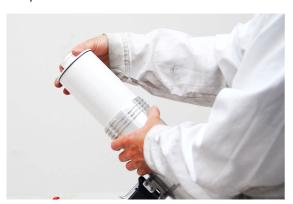
The cartridge can now be filled manually or with the HAMA plastering machine. Then place the complete cartridge in the repair gun.
