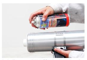
Apply silicone spray (108401BP032) to the repair gun's screw threads, where the black union nut is attached.
