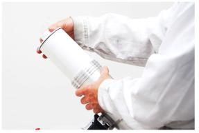
Now remove the cartridge (108401BP001) from the repair gun.
