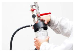
Fit the black union nut (108401PA003), including the spray section, on the repair gun.
