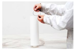
Take a new cartridge (108401BP001) and fit the supplied O-ring (108401BP003) around the cartridge.
