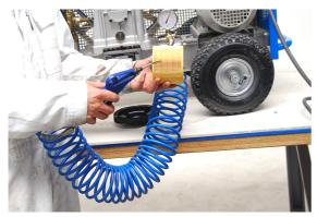
Connect an air gun to the air hose or directly to the compressor and blow the air filter clean.
