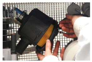
Fit the air filter (2012666) back in place and screw the cover back onto the air filter housing.
